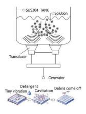
Ultrasonic cleaning is on based on the cavitation effect caused by high-frequency ultrasonic wave vibration signal in the fluid. Microscopic bubbles are formed, and they implode violently causing the cavitation which creates an intense scrubbing action on the surface of the item being cleaned. The bubbles are small enough to penetrate microscopic crevices, cleaning them thoroughly and consistently.
